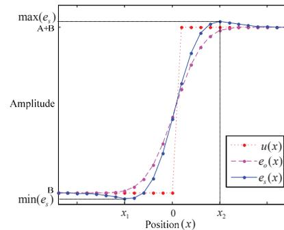
Fig. 2. Signal model for three kinds of step edge.  $u(x)$ : the ideal step edge;  $e_o(x)$ : the natural step edge in unsharpened images;  $e_s(x)$ : the sharpened step edge in sharpened images.
